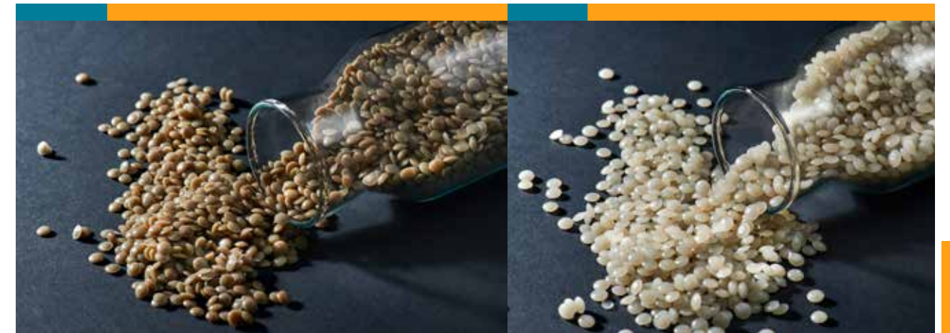
Natural Granules It is generally obtained from clean, unprinted transparent wastes obtained from factory.
